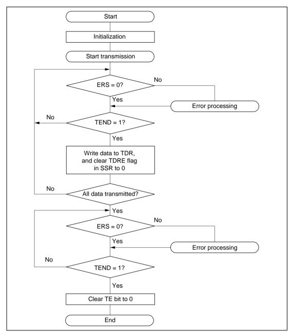
Figure 13.4 Example of Transmission Processing Flow
