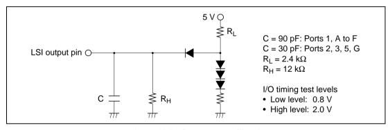
Figure 19.3 Output Load Circuit
