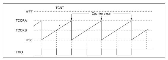
Figure 10.9 Example of Pulse Output
