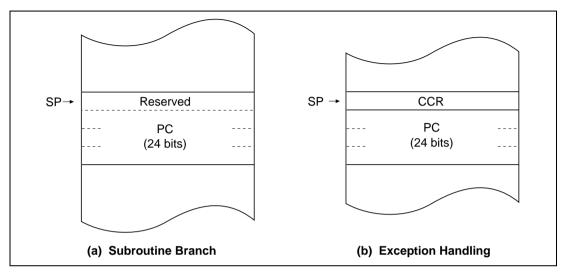
Figure 2.5 Stack Structure in Advanced Mode
