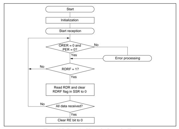
Figure 13.7 Example of Reception Processing Flow
