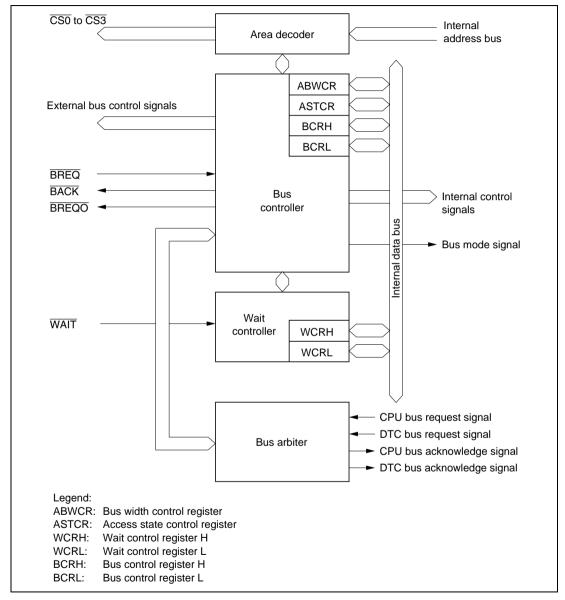
Figure 6.1 Block Diagram of Bus Controller
