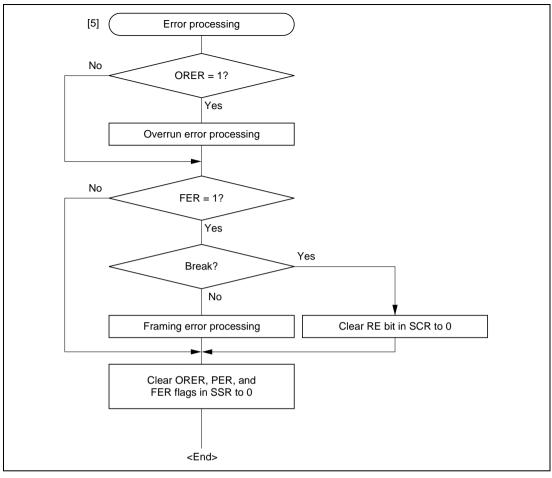
Figure 12.12 Sample Multiprocessor Serial Reception Flowchart (cont)
