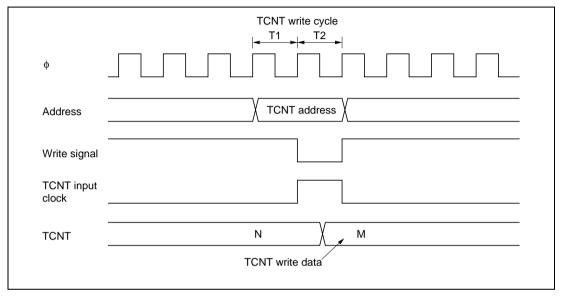
Figure 9.46 Contention between TCNT Write and Increment Operations
