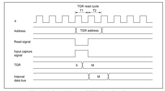
Figure 9.49 Contention between TGR Read and Input Capture
