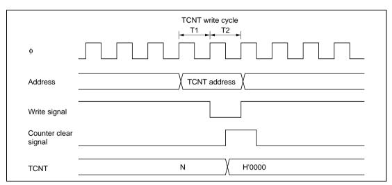
Figure 9.45 Contention between TCNT Write and Clear Operations
