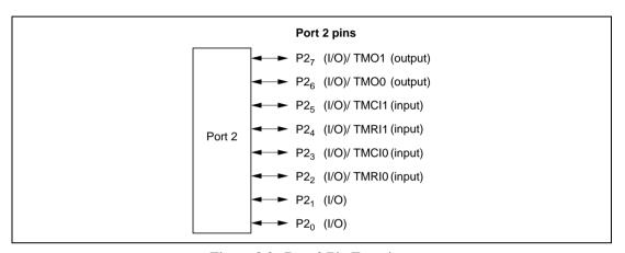
Figure 8.2 Port 2 Pin Functions
