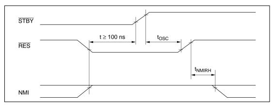
Figure F.2 Timing of Recovery from Hardware Standby Mode
