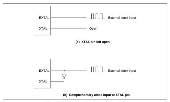
Figure 17.5 External Clock Input (Examples)
