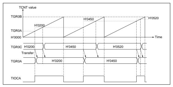
Figure 9.19 Example of Buffer Operation (1)
