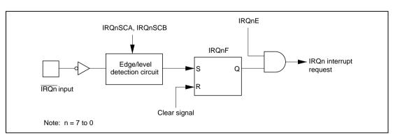
Figure 5.2 Block Diagram of Interrupts IRQ7 to IRQ0
