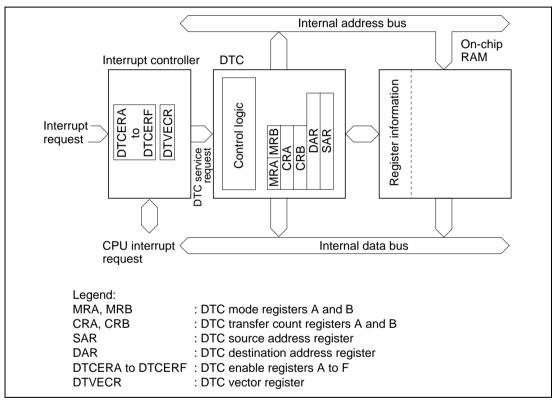
Figure 7.1 Block Diagram of DTC
