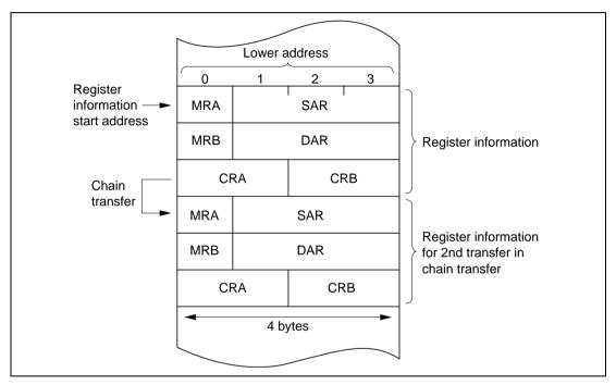
Figure 7.5 Location of DTC Register Information in Address Space
