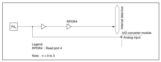
Figure C.4 Port 4 Block Diagram (Pins P4<sub>0</sub> to P4<sub>3</sub>)
