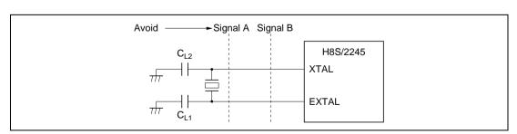
Figure 17.4 Example of Incorrect Board Design
