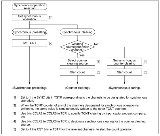
Figure 9.14 Example of Synchronous Operation Setting Procedure
