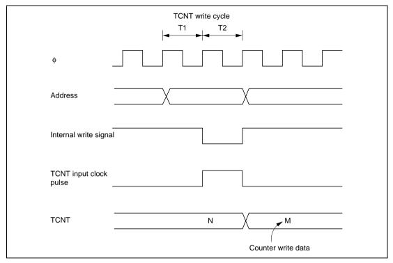
Figure 11.8 Contention between TCNT Write and Increment
