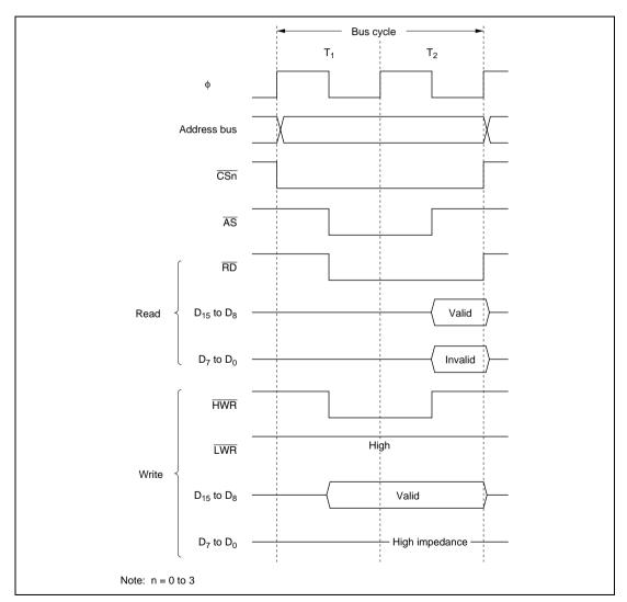
Figure 6.10 Bus Timing for 8-Bit 2-State Access Space
