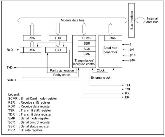
Figure 12.1 Block Diagram of SCI
