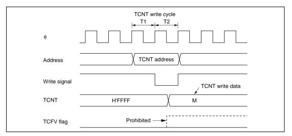
Figure 9.53 Contention between TCNT Write and Overflow
