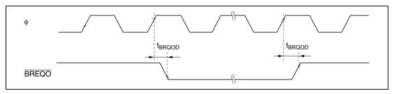
Figure 19.14 External Bus Request Output Timing
