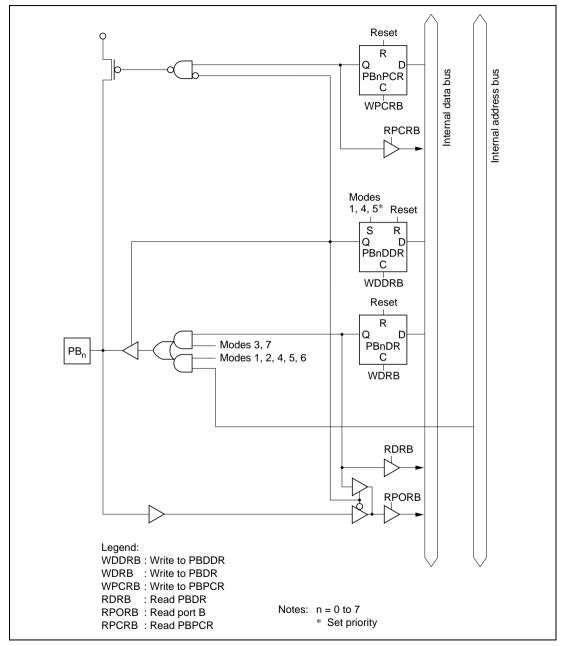
Figure C.7 Port B Block Diagram (Pins PB<sub>0</sub> to PB<sub>7</sub>)
