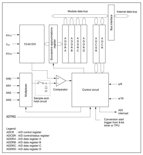
Figure 14.1 Block Diagram of A/D Converter
