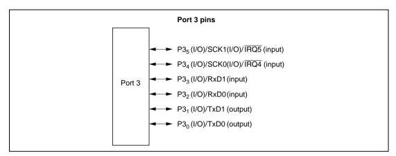
Figure 8.3 Port 3 Pin Functions
