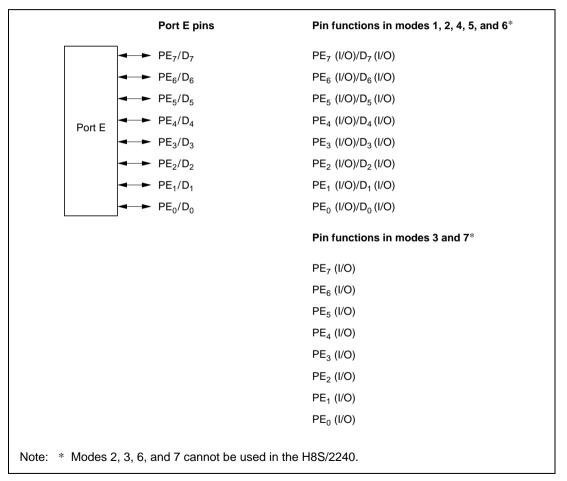
**Figure 8.21 Port E Pin Functions**
