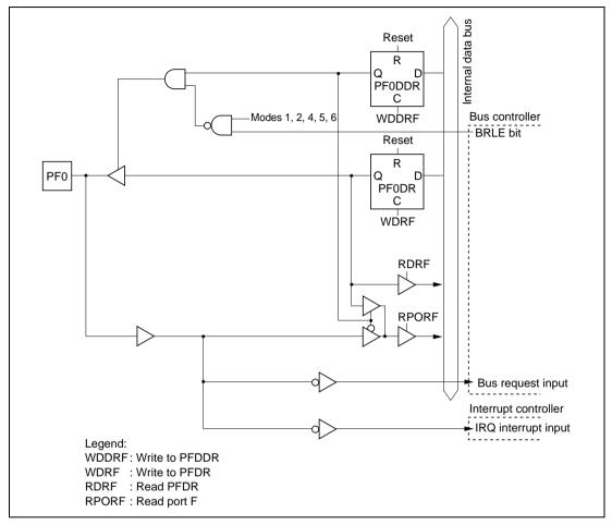
Figure C.11 (a) Port F Block Diagram (Pin PF<sub>0</sub>)
