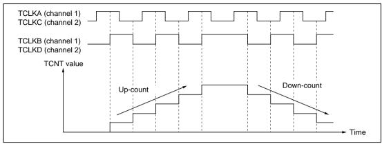
Figure 9.29 Example of Phase Counting Mode 4 Operation
