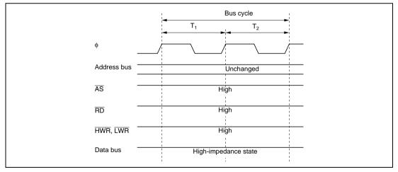
Figure 6.7 Pin States during On-Chip Peripheral Module Access
