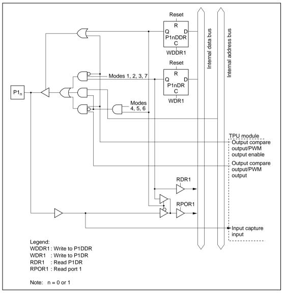
Figure C.1 (a) Port 1 Block Diagram (Pins P1, and P1,)
