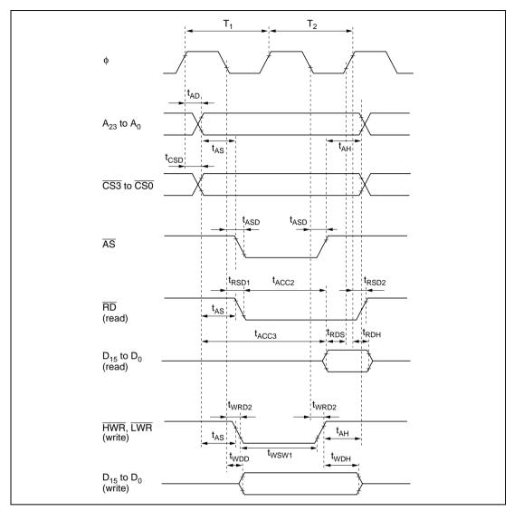
Figure 19.8 Basic Bus Timing (Two-State Access)
