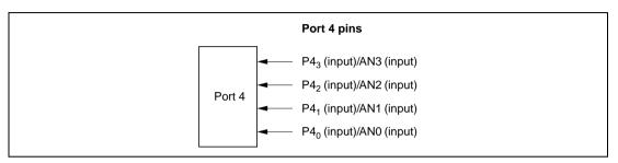
**Figure 8.4 Port 4 Pin Functions**
