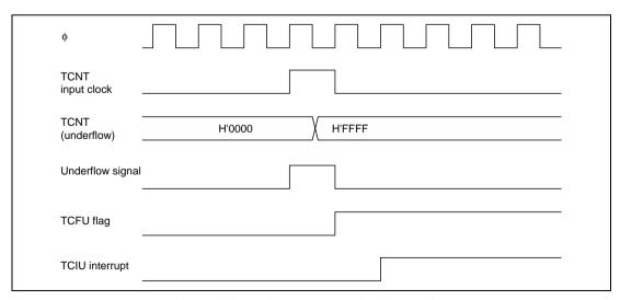
Figure 9.41 TCIU Interrupt Setting Timing
