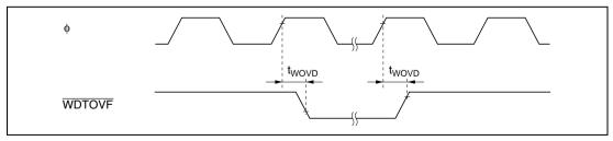
Figure 19.21 WDT Output Timing
