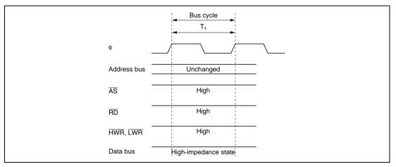
Figure 6.5 Pin States during On-Chip Memory Access
