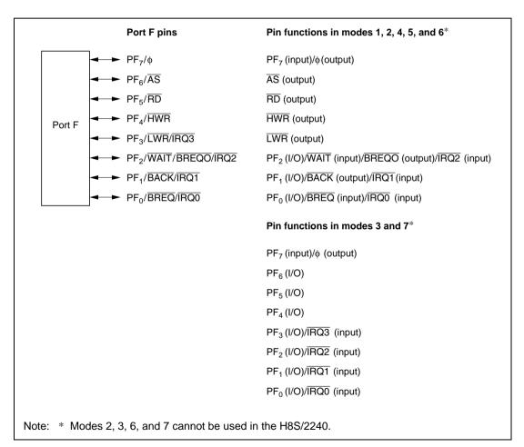
Figure 8.24 Port F Pin Functions
