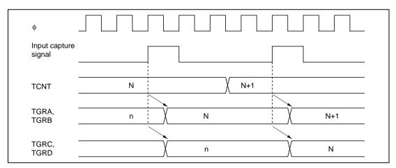
Figure 9.37 Buffer Operation Timing (Input Capture)
