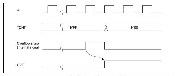
Figure 11.6 Timing of Setting of OVF
