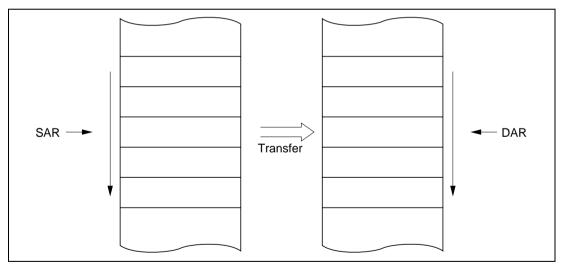
Figure 7.6 Memory Mapping in Normal Mode
