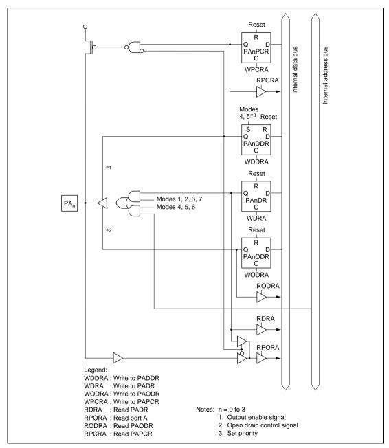
Figure C.6 Port A Block Diagram (Pins PA<sub>0</sub> to PA<sub>3</sub>)
