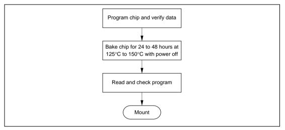
Figure 16.6 Recommended Screening Procedure
