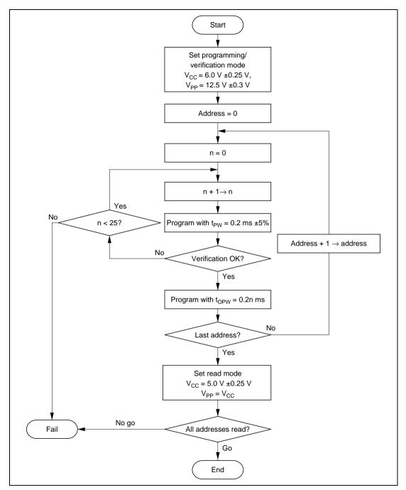
Figure 16.4 High-Speed Programming Flowchart
