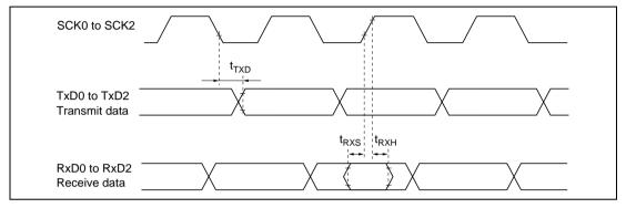
Figure 19.23 SCI Input/Output Timing Synchronous Mode
