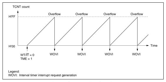
Figure 11.5 Interval Timer Operation
