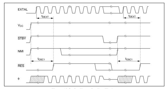
Figure 19.5 Oscillator Settling Timing
