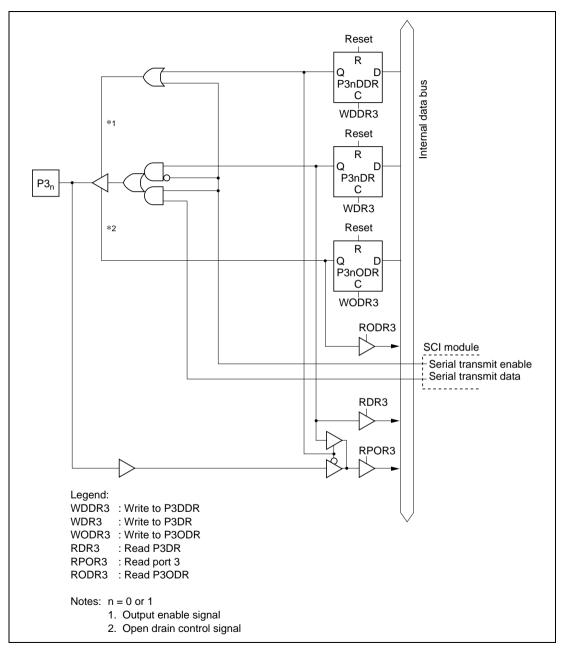
Figure C.3 (a) Port 3 Block Diagram (Pins P3, and P3,)
