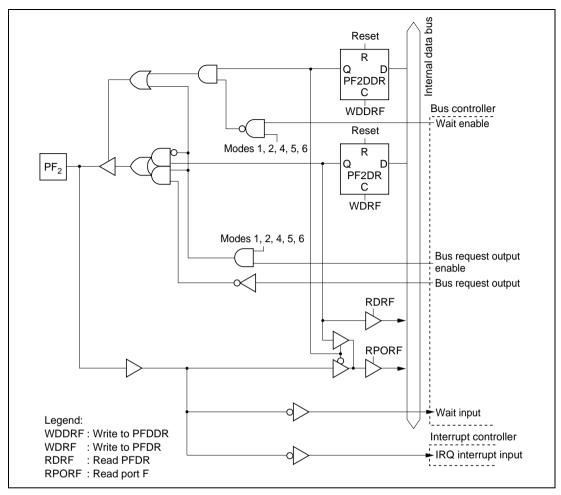
Figure C.11 (c) Port F Block Diagram (Pin PF<sub>2</sub>)
