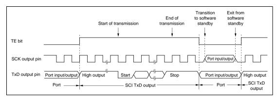
Figure 12.24 Asynchronous Transmission Using Internal Clock
