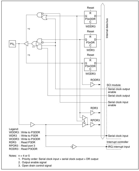
Figure C.3 (c) Port 3 Block Diagram (Pins P3, and P3,
