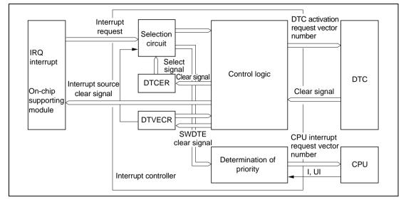
Figure 5.10 Interrupt Control for DTC
