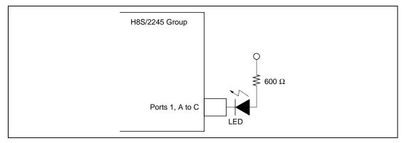
Figure 19.2 LED Drive Circuit (Example)
