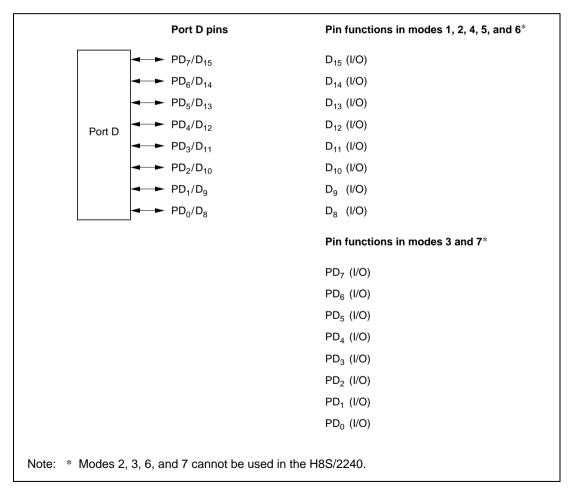
**Figure 8.18 Port D Pin Functions**
