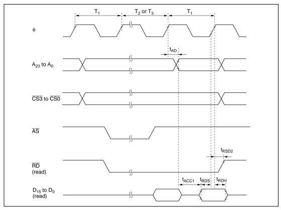
Figure 19.12 Burst ROM Access Timing (One-State Access)
