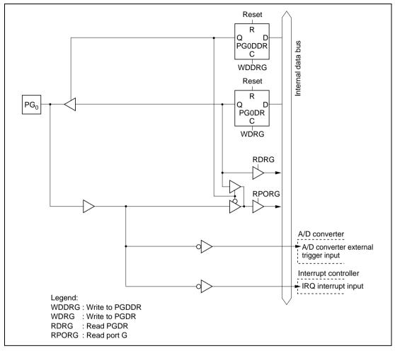
Figure C.12 (a) Port G Block Diagram (Pin  $PG_0$ )
