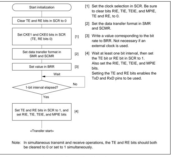
Figure 12.15 Sample SCI Initialization Flowchart
