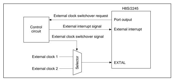
Figure 17.7 Sample External Clock Switching Circuit
