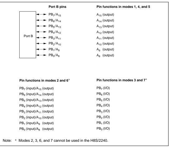
Figure 8.10 Port B Pin Functions
