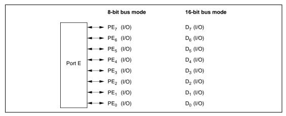
Figure 8.22 Port E Pin Functions (Modes 1, 2, 4, 5, and 6)
