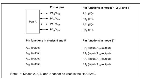
Figure 8.6 Port A Pin Functions
