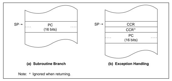
Figure 2.3 Stack Structure in Normal Mode
