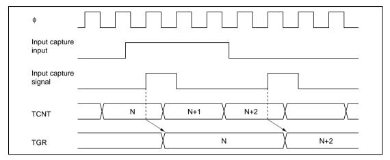
Figure 9.33 Input Capture Input Signal Timing
