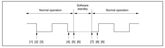
Figure 13.9 Clock Halt and Restart Procedure
