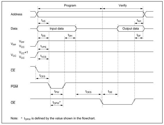
Figure 16.5 PROM Programming/Verification Timing
