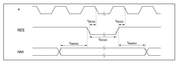
Figure 19.6 Reset Input Timing
