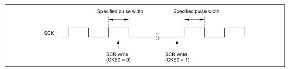
Figure 13.8 Timing for Fixing Clock Output Level
