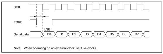
Figure 12.22 Example of Clocked Synchronous Transmission by DTC
