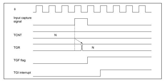
Figure 9.39 TGI Interrupt Timing (Input Capture)
