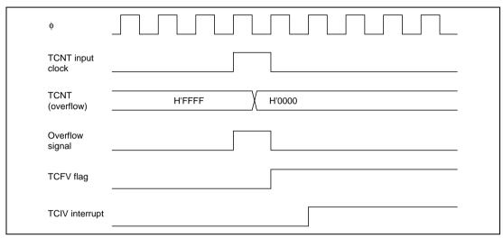
Figure 9.40 TCIV Interrupt Setting Timing
