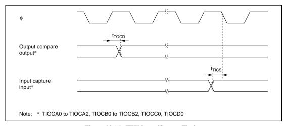
Figure 19.16 TPU Input/Output Timing
