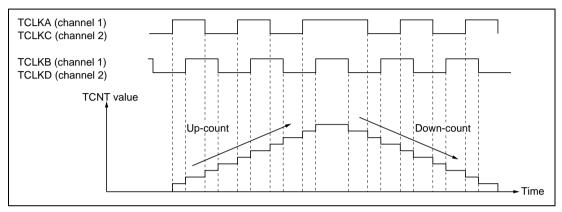
Figure 9.26 Example of Phase Counting Mode 1 Operation
