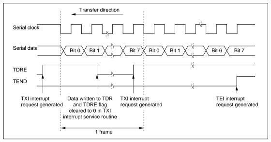
Figure 12.17 Example of SCI Operation in Transmission
