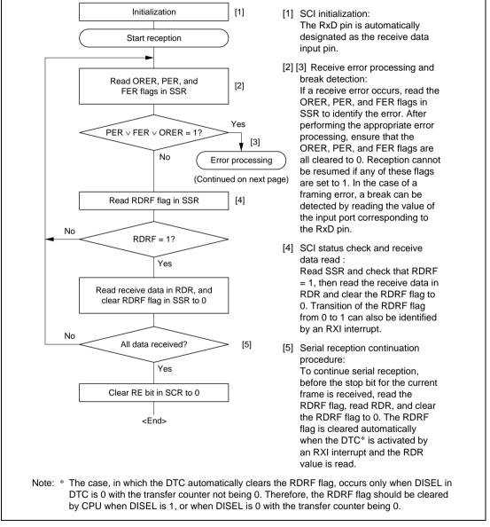
Figure 12.7 Sample Serial Reception Data Flowchart
