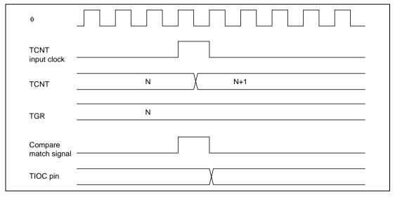
Figure 9.32 Output Compare Output Timing
