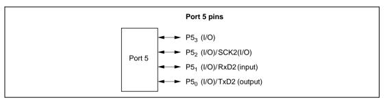
Figure 8.5 Port 5 Pin Functions
