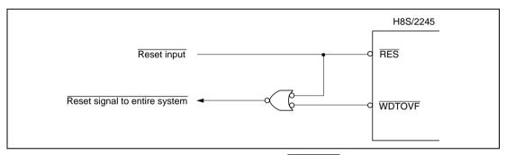
Figure 11.9 Circuit for System Reset by WDTOVF Signal (Example)
