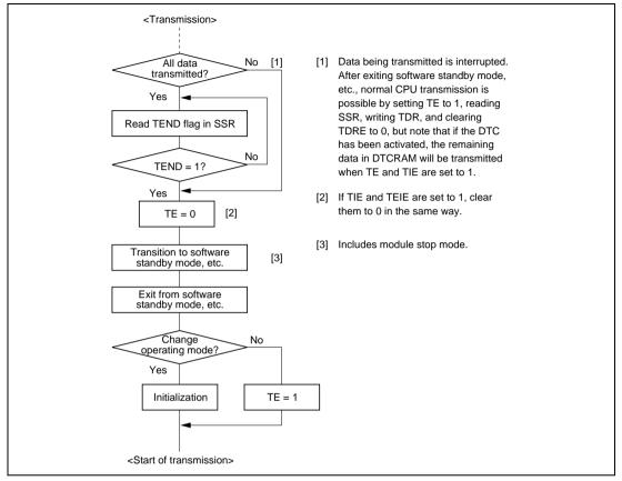
Figure 12.23 Sample Flowchart for Mode Transition during Transmission
