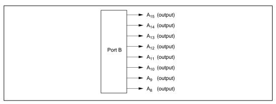
Figure 8.11 Port B Pin Functions (Modes 1, 4, and 5)
