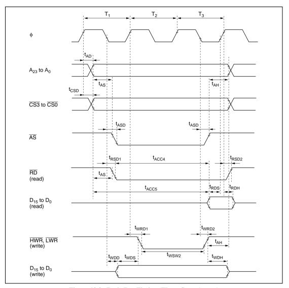
Figure 19.9 Basic Bus Timing (Three-State Access)
