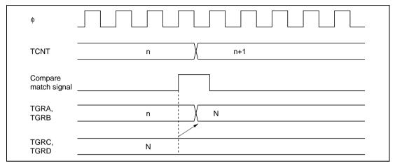
**Figure 9.36 Buffer Operation Timing (Compare Match)**
