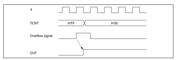
Figure 10.8 Timing of OVF Setting
