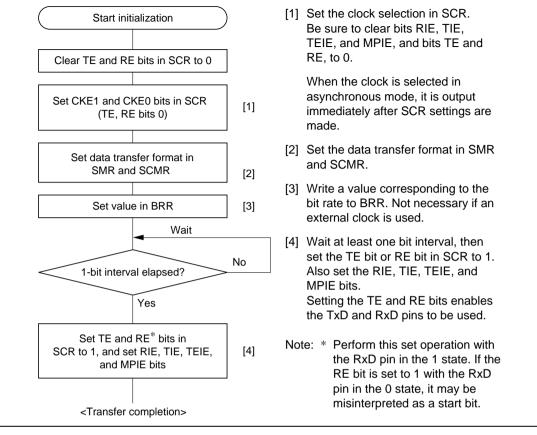
Figure 12.4 Sample SCI Initialization Flowchart
