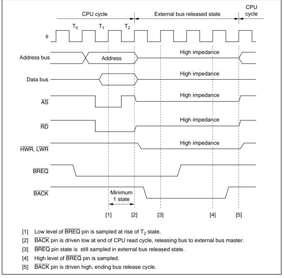
Figure 6.23 Bus-Released State Transition Timing
