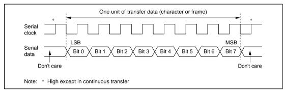
Figure 12.14 Data Format in Synchronous Communication
