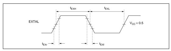
Figure 17.6 External Clock Input Timing
