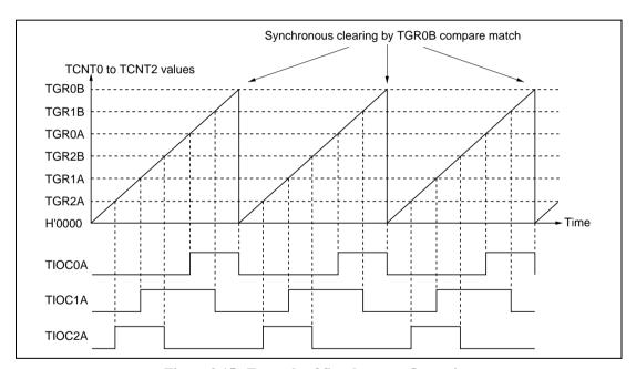
Figure 9.15 Example of Synchronous Operation
