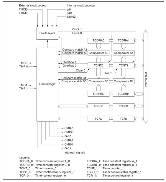
Figure 10.1 Block Diagram of 8-Bit Timer
