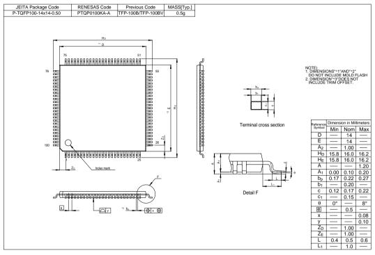
Figure H.2 TFP-100B Package Dimensions
