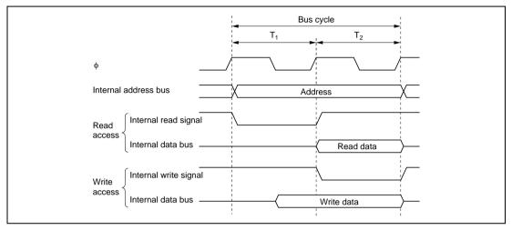
Figure 6.6 On-Chip Peripheral Module Access Cycle
