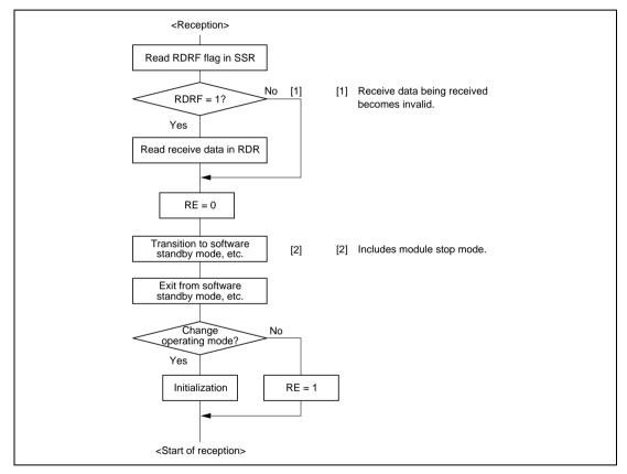
Figure 12.26 Sample Flowchart for Mode Transition during Reception
