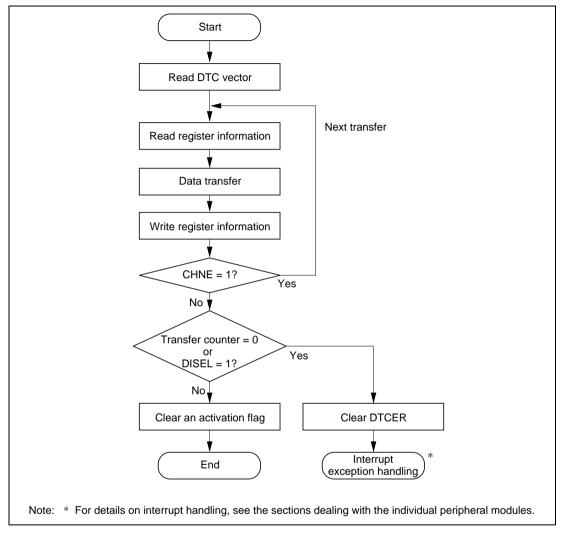
Figure 7.2 Flowchart of DTC Operation
