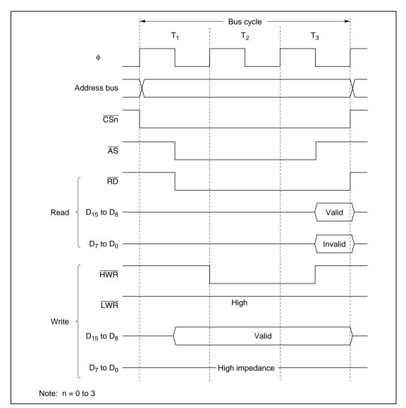
Figure 6.11 Bus Timing for 8-Bit 3-State Access Space
