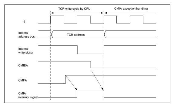
Figure 5.9 Contention between Interrupt Generation and Disabling
