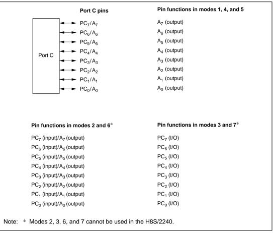
**Figure 8.14 Port C Pin Functions**
