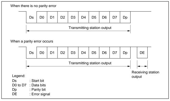
Figure 13.3 Smart Card Interface Data Format
