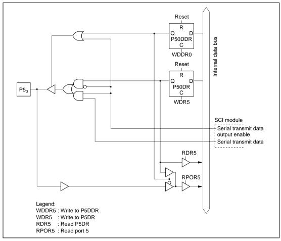
Figure C.5 (a) Port 5 Block Diagram (Pin P5<sub>0</sub>)
