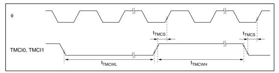
Figure 19.19 8-Bit Timer Clock Input Timing
