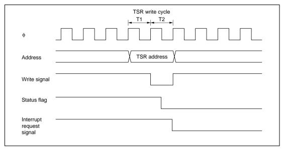
Figure 9.42 Timing for Status Flag Clearing by CPU
