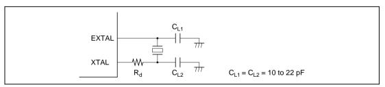
Figure 17.2 Connection of Crystal Resonator (Example)
