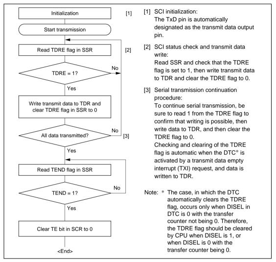
Figure 12.16 Sample Serial Transmission Flowchart
