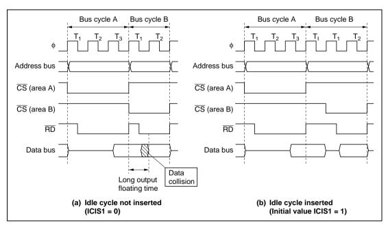
Figure 6.20 Example of Idle Cycle Operation (1)
