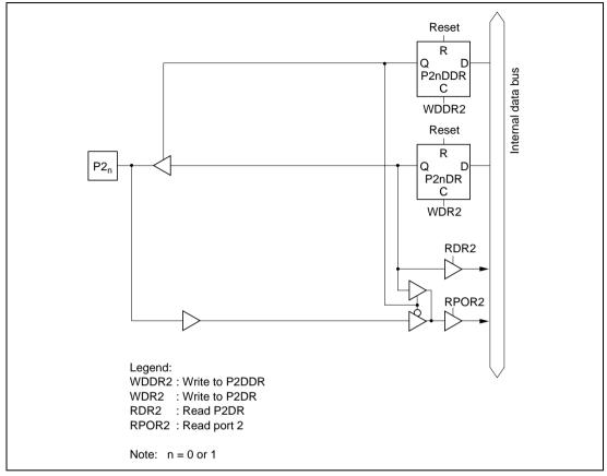
Figure C.2 (a) Port 2 Block Diagram (Pins P2, and P2,)
