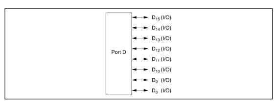
Figure 8.19 Port D Pin Functions (Modes 1, 2, 4, 5, and 6)
