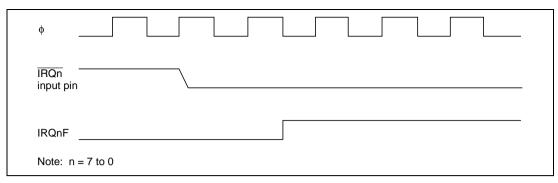
Figure 5.3 Timing of Setting IRQnF
