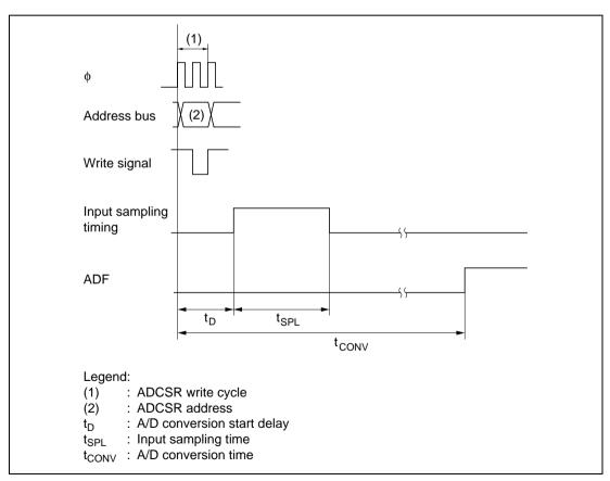
Figure 14.5 A/D Conversion Timing
