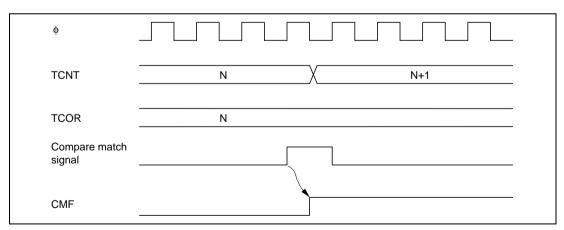
Figure 10.4 Timing of CMF Setting
