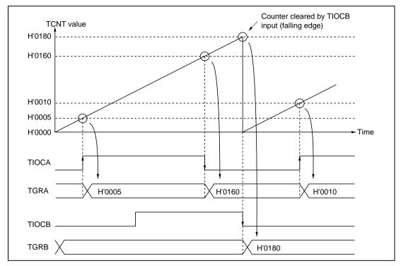
Figure 9.13 Example of Input Capture Operation
