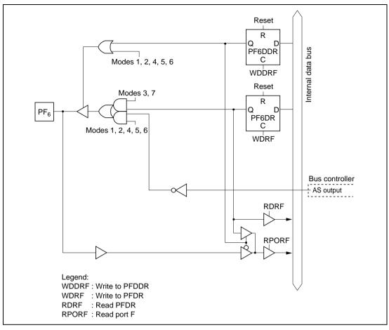
Figure C.11 (g) Port F Block Diagram (Pin  $PF_6$ )
