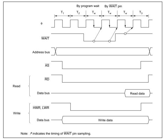
Figure 6.18 Example of Wait State Insertion Timing
