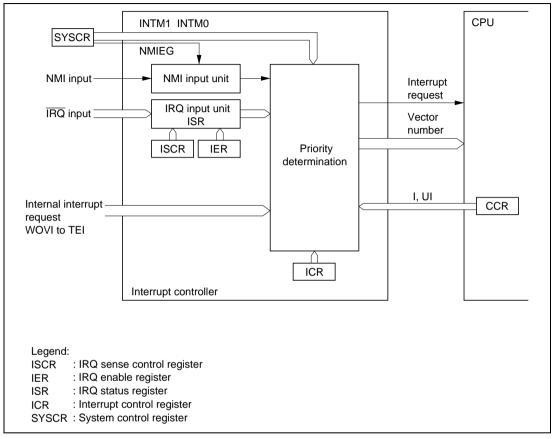
Figure 5.1 Block Diagram of Interrupt Controller
