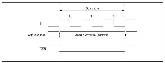
Figure 6.3  $\overline{CSn}$  Signal Output Timing (n = 0 to 3)
