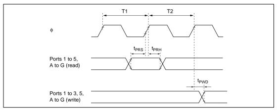
Figure 19.15 I/O Port Input/Output Timing
