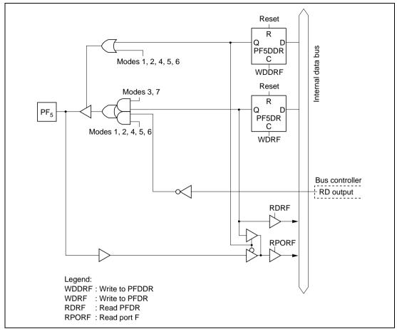
Figure C.11 (f) Port F Block Diagram (Pin  $PF_s$ )
