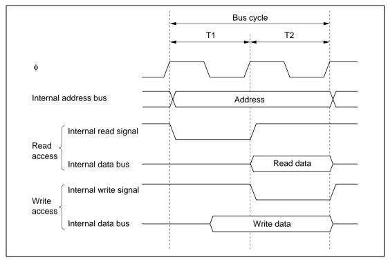
Figure 2.19 On-Chip Supporting Module Access Cycle
