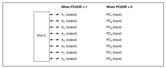
Figure 8.16 Port C Pin Functions (Modes 2 and 6)
