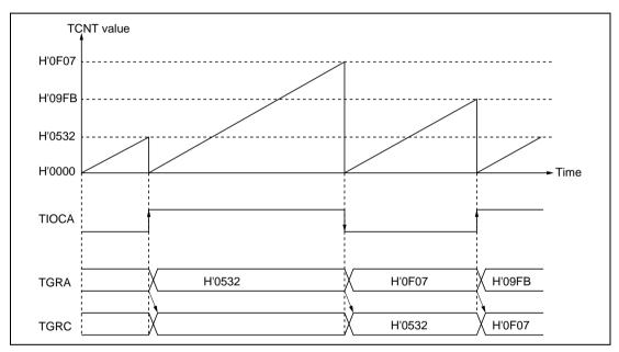
Figure 9.20 Example of Buffer Operation (2)
