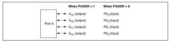
Figure 8.9 Port A Pin Functions (Mode 6)
