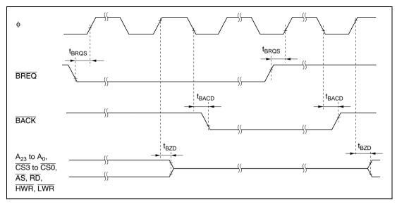
Figure 19.13 External Bus Release Timing
