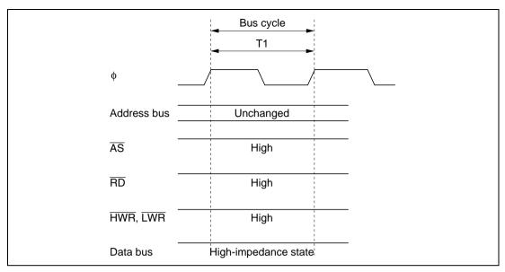
Figure 2.18 Pin States during On-Chip Memory Access
