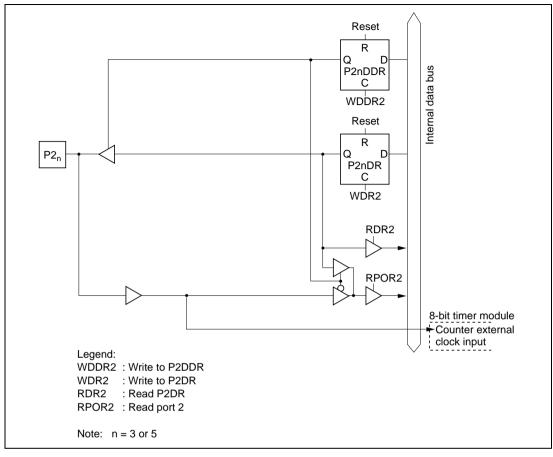
Figure C.2 (c) Port 2 Block Diagram (Pins P2, and P2,
