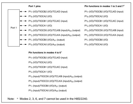
**Figure 8.1 Port 1 Pin Functions**
