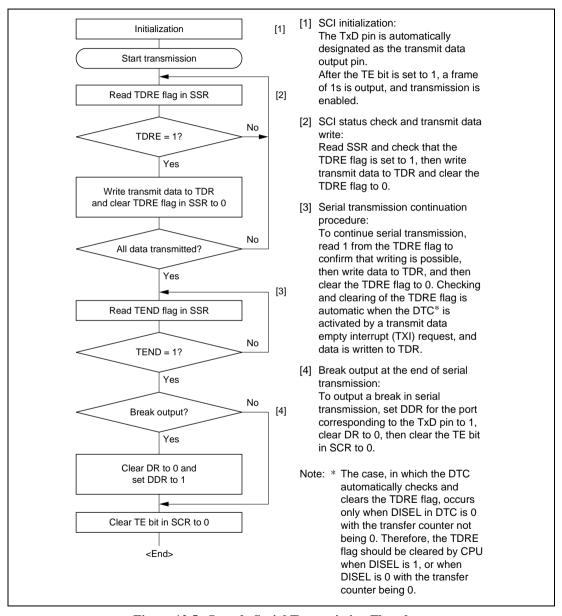
Figure 12.5 Sample Serial Transmission Flowchart
