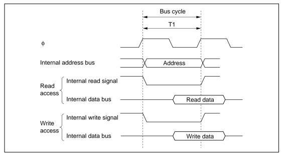
Figure 2.17 On-Chip Memory Access Cycle
