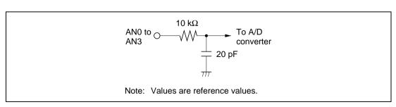
Figure 14.8 Analog Input Pin Equivalent Circuit
