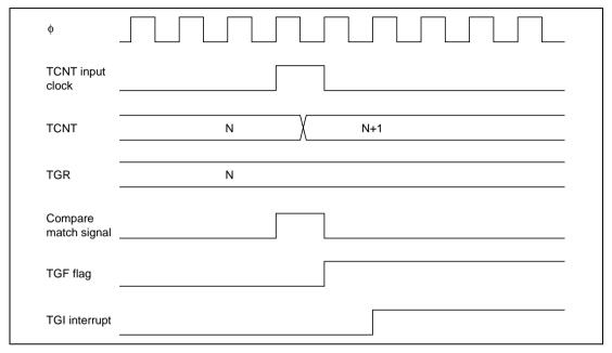
**Figure 9.38 TGI Interrupt Timing (Compare Match)**
