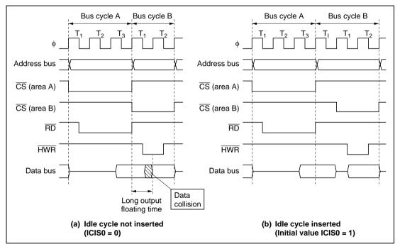
Figure 6.21 Example of Idle Cycle Operation (2)
