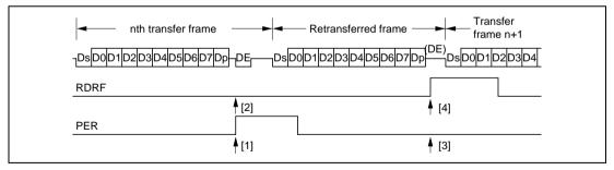
Figure 13.11 Retransfer Operation in SCI Receive Mode
