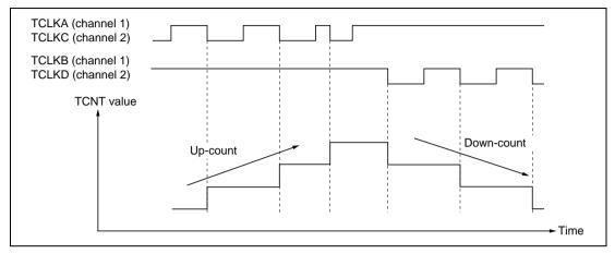
Figure 9.28 Example of Phase Counting Mode 3 Operation
