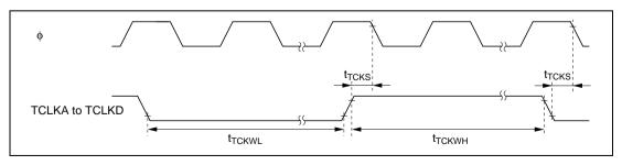
Figure 19.17 TPU Clock Input Timing
