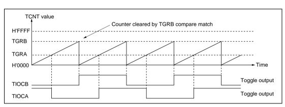
Figure 9.11 Example of Toggle Output Operation
