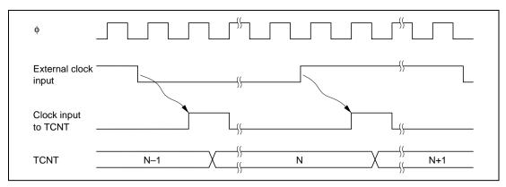
Figure 10.3 Count Timing for External Clock Input
