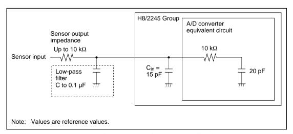
Figure 14.11 Example of Analog Input Circuit
