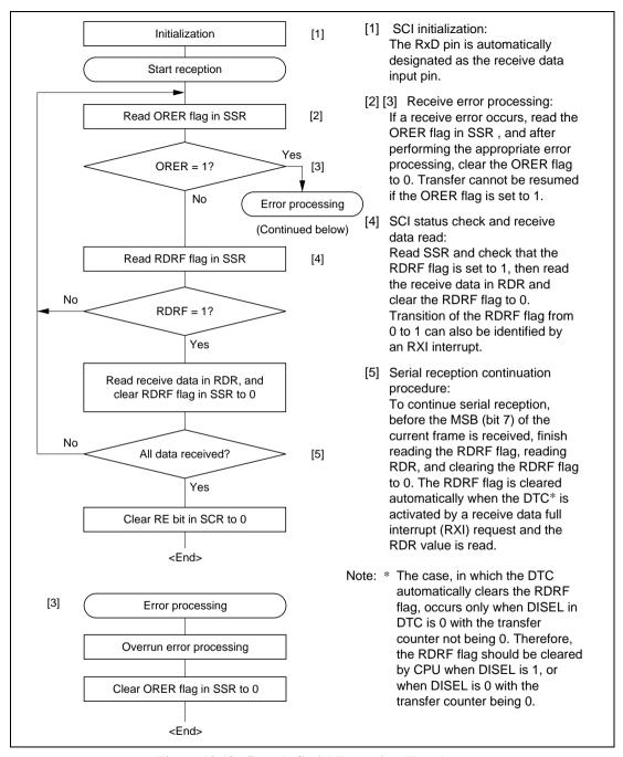
Figure 12.18 Sample Serial Reception Flowchart
