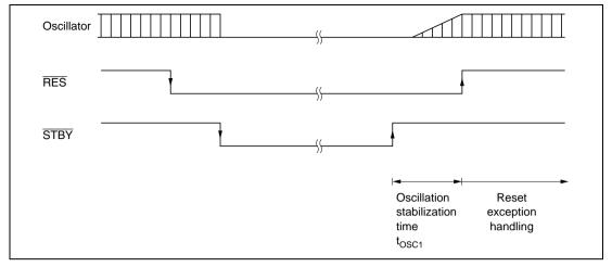
Figure 18.3 Hardware Standby Mode Timing (Example)
