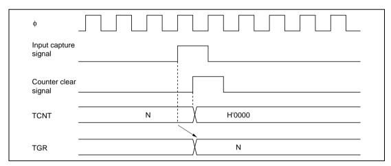
Figure 9.35 Counter Clear Timing (Input Capture)
