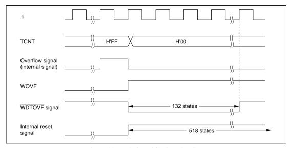
Figure 11.7 Timing of Setting of WOVF
