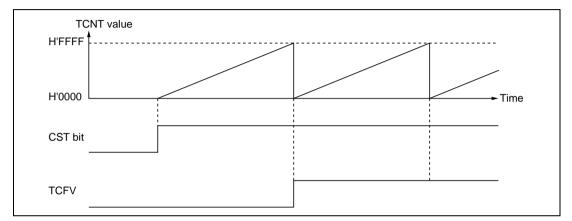
Figure 9.7 Free-Running Counter Operation
