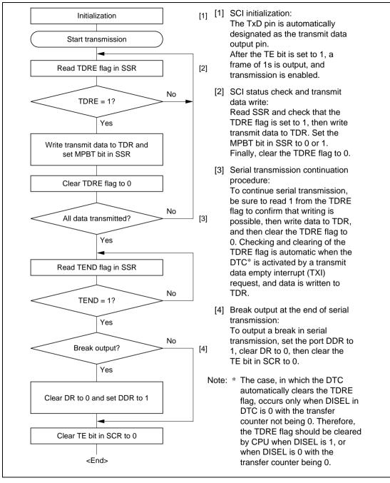
Figure 12.10 Sample Multiprocessor Serial Transmission Flowchart
