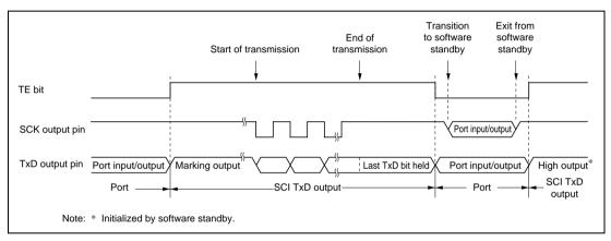
Figure 12.25 Synchronous Transmission Using Internal Clock
