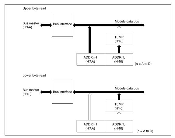
Figure 14.2 ADDR Access Operation (Reading H'AA40)
