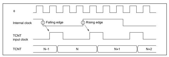
Figure 9.30 Count Timing in Internal Clock Operation
