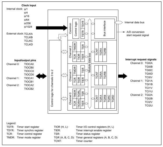
Figure 9.1 Block Diagram of TPU
