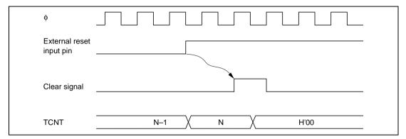
Figure 10.7 Timing of External Reset
