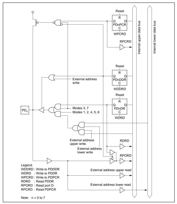
Figure C.9 Port D Block Diagram (Pins PD, to PD,)
