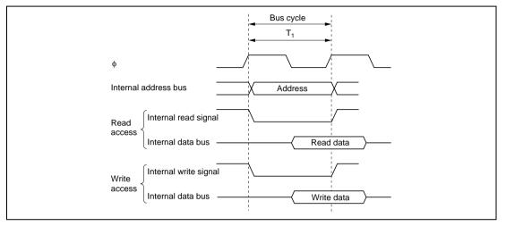
Figure 6.4 On-Chip Memory Access Cycle
