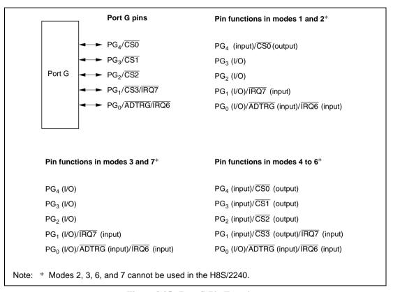
Figure 8.25 Port G Pin Functions
