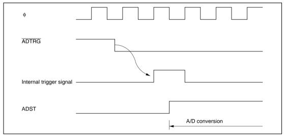
Figure 14.6 External Trigger Input Timing
