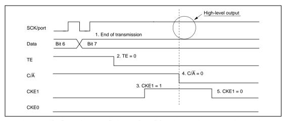
Figure 12.28 Operation when Switching from SCK Pin Function to Port Pin Function (Example of Preventing Low-Level Output)
