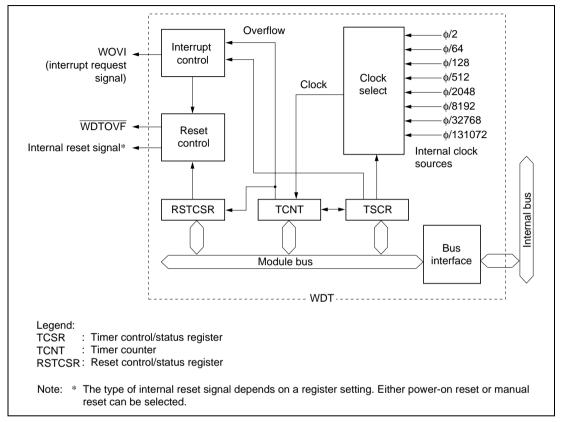
Figure 11.1 Block Diagram of WDT
