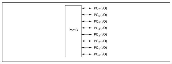
Figure 8.17 Port C Pin Functions (Modes 3 and 7)
