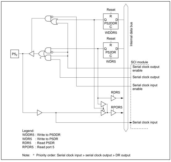
Figure C.5 (c) Port 5 Block Diagram (Pin P5<sub>2</sub>)
