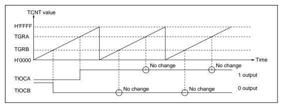
Figure 9.10 Example of 0 Output/1 Output Operation
