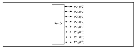
Figure 8.20 Port D Pin Functions (Modes 3 and 7)
