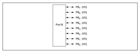
Figure 8.13 Port B Pin Functions (Modes 3 and 7)
