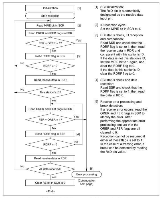
Figure 12.12 Sample Multiprocessor Serial Reception Flowchart
