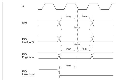
Figure 19.7 Interrupt Input Timing
