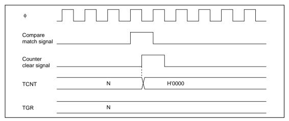
Figure 9.34 Counter Clear Timing (Compare Match)
