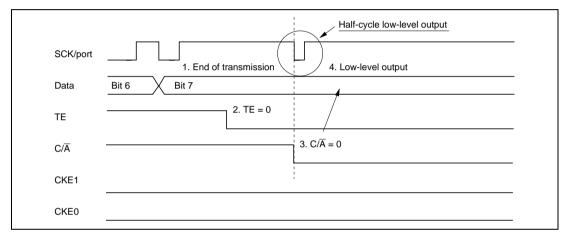
Figure 12.27 Operation when Switching from SCK Pin Function to Port Pin Function
