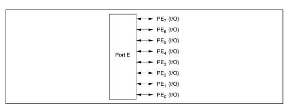
Figure 8.23 Port E Pin Functions (Modes 3 and 7)
