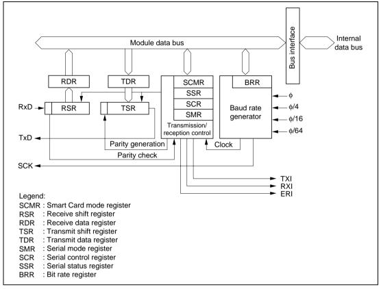
Figure 13.1 Block Diagram of Smart Card Interface
