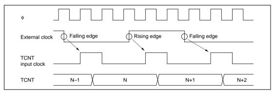
Figure 9.31 Count Timing in External Clock Operation
