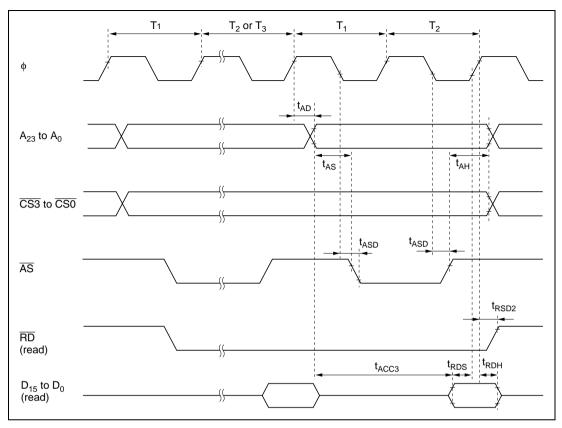
Figure 19.11 Burst ROM Access Timing (Two-State Access)
