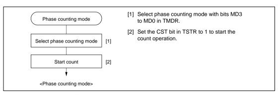
Figure 9.25 Example of Phase Counting Mode Setting Procedure
