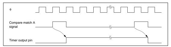
Figure 10.5 Timing of Timer Output
